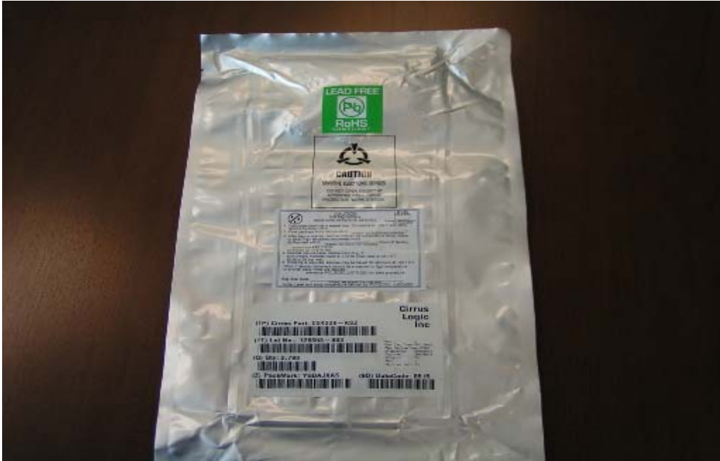
Example of Moisture Barrier Bag with RoHS label placement
