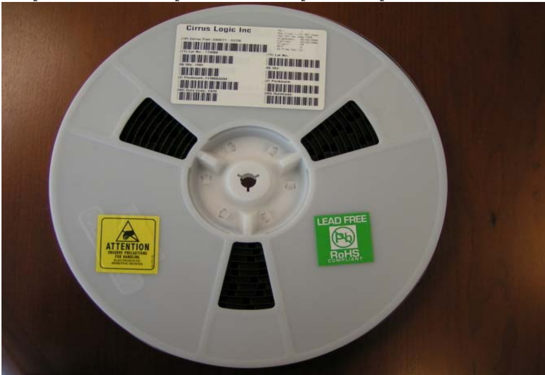
Example of RoHS label placement for Tape & Reel products
